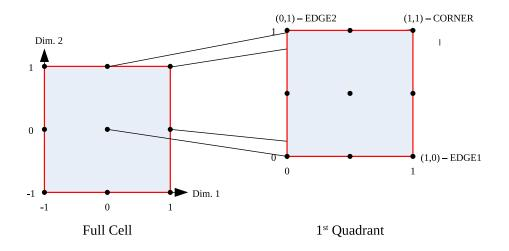
Figure 18: An example of specifying 2D stagger locations using coordinates.
